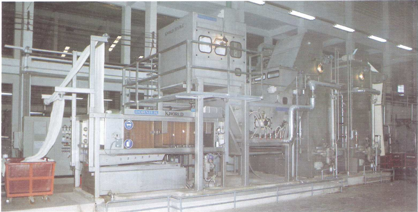
Combined mercerising- and bleaching range type CMB in operation
